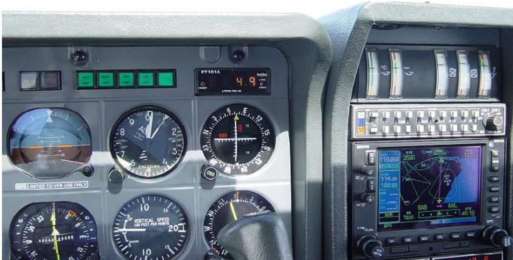
The GNS530 and the now defunct VFR Only Placard (below the AI)
