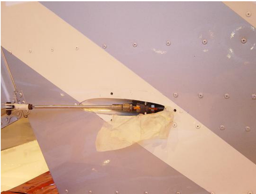
The source of my Rudder trim problems - the two orange nuts had started to come adrift
