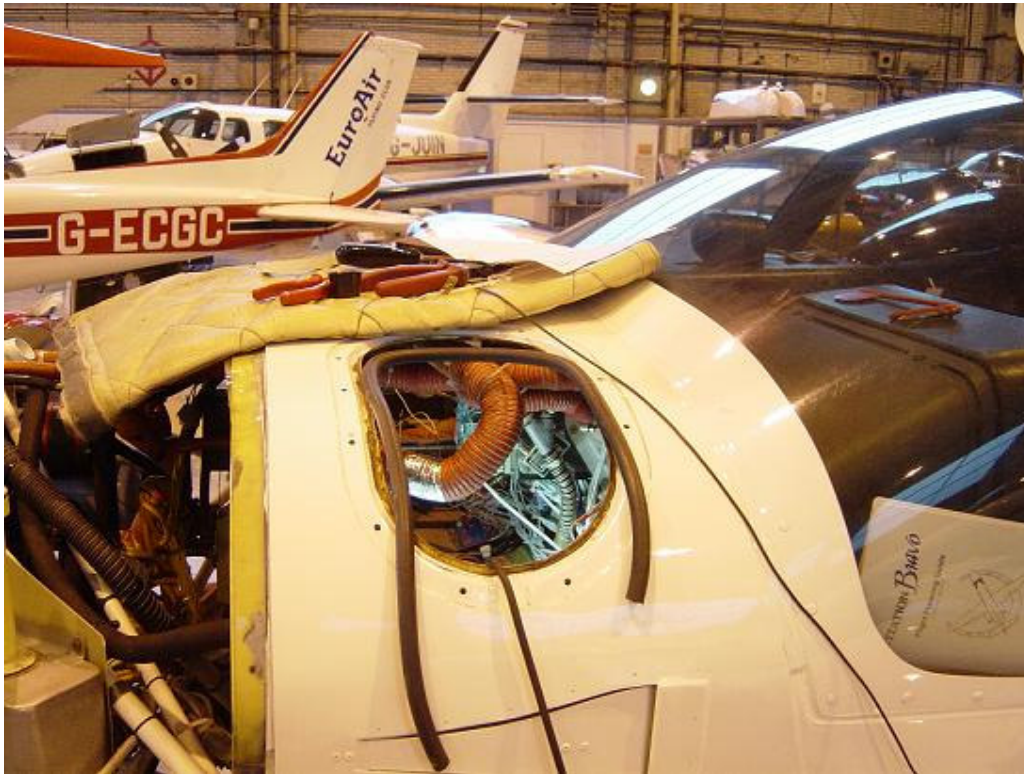
Work in progress on the installation of my Air Data Computer
